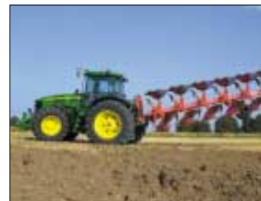
Choose your rear 3-point hitch: The standard 3-point hitch features 11350 kg max. lift capacity. For heavier mounted implements, you can opt for a 8150 kg max. 3-point hitch. Both feature full electronic load and depth adjustment for precise implement placement.
